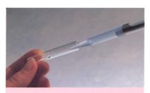
Add 0.4ml Oxoid Extraction Enzyme to the test tube.
