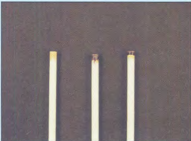
Oxidase test using Oxoid Touchsticks code BR64. Left: Negative test. Centre and right: Positive test.
