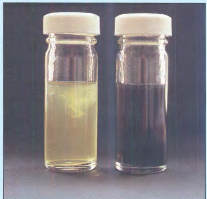
Hydrogen sulphide production. Left: Negative test. Right: Positive test showing blackening of FBP medium caused by production of hydrogen sulphide.
