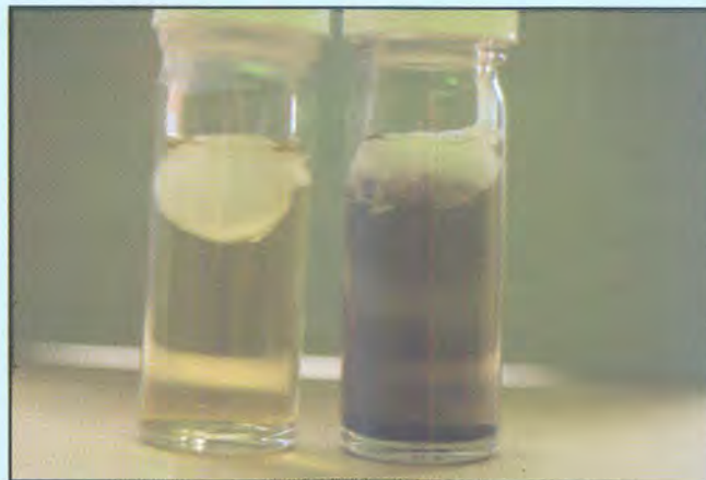
Appearance of Staph. aureus culture in Giolitti-Cantoni broth (right). Uninoculated medium on the left. The surface of the medium is sealed with paraffin wax to create anaerobic growth conditions.
